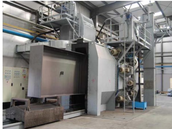
12 Wheel Shot Blasting Machine for 2m high x 0.8m wide Product
